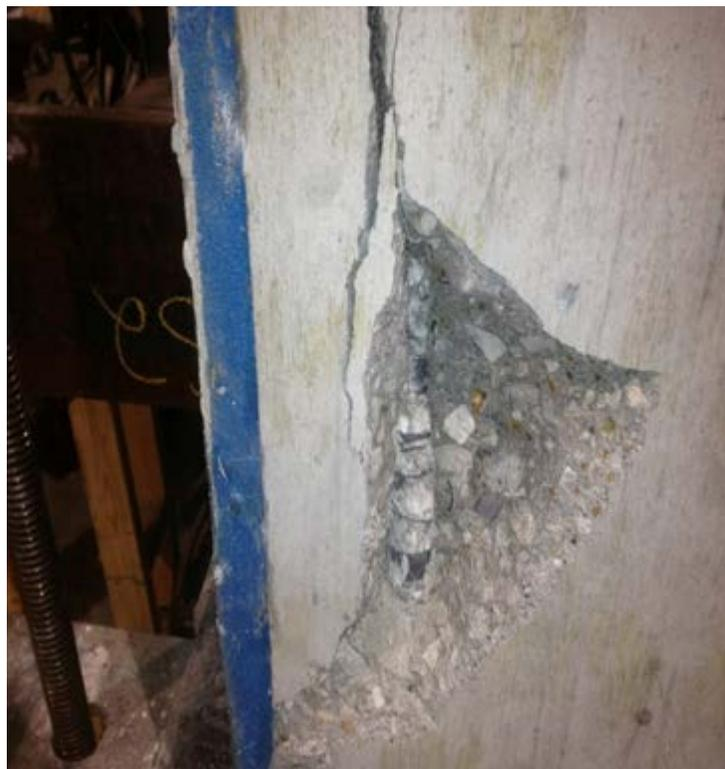
**Figure 3.6** Tail kickout (TK) failure
