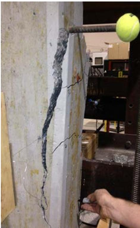
**Figure 3.4** Side splitting (SS) failure
