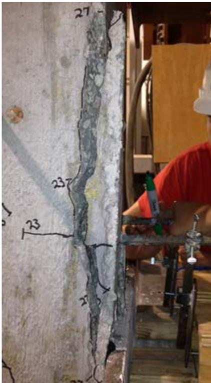
**Figure 3.2** Front pullout (FP) failure
