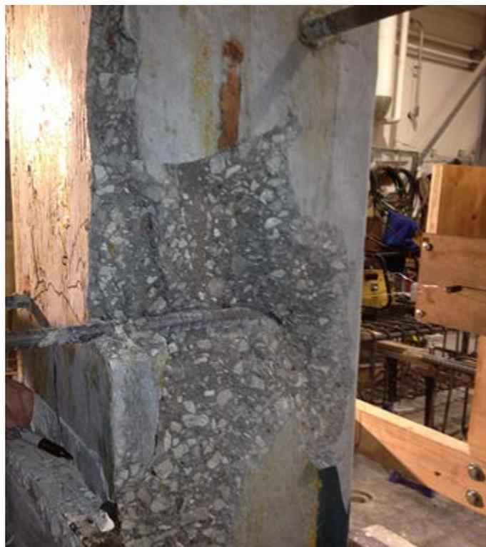
**Figure 3.5** Side blowout (SB) failure
