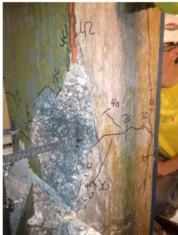
**Figure 3.3** Front blowout (FB) failure
