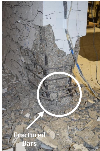
Figure 79 – Wall T4 with bar fracture in confined stem during second cycle to 4% drift ratio (stem in tension)
