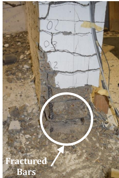
Figure 73 – Wall T1 with bar fracture in confined stem during first cycle to 4% drift ratio (stem in tension)
