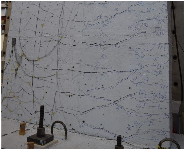
Figure 67 – Wall T4 without bar buckling or fracture in unconfined flange during second cycle to 2% drift ratio (stem in compression)
