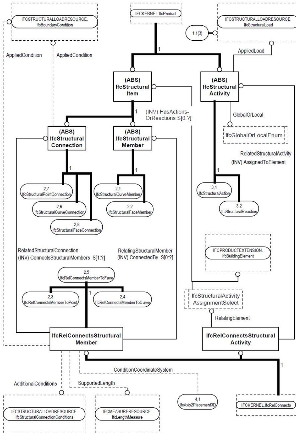
FIGURE 2 EXPRESS G diagram showing the inheritance structure and main relationships and attributes defined in the structural analysis model.
